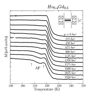
FIG. 1. Mutual inductance M vs T dependences at different pressures. Pressures are indicated on the curves. Curves are shifted vertically for clarity, onsets omitted. Arrows indicate antiferromagnetic area. Inset: sketch of the experiment.
